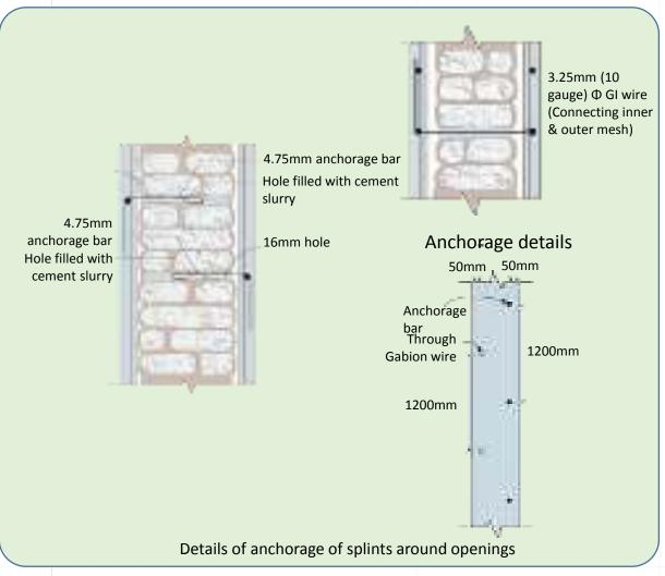
Option 2: Provide Welded GI wire mesh splint on outer faces of wall wherever required and anchor them sufficiently with the wall.
