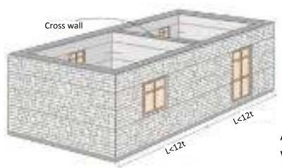
Addition of cross wall when length of wall is greater than 12t.
