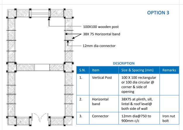
FLOOR PLAN (STONE MASONRY)
