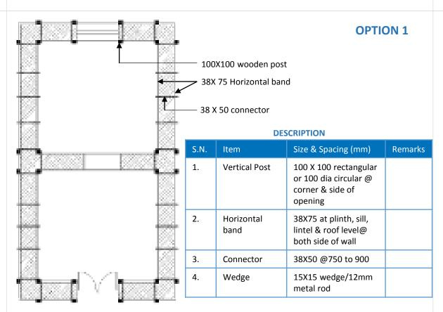
FLOOR PLAN (STONE MASONRY)
